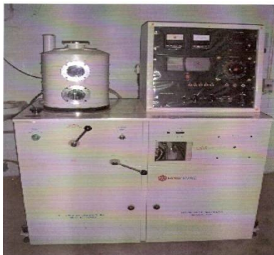
Figure 4: HINDHIVAC Vacuum Coater
